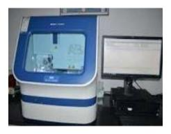
The 3500 or 3500xL analyzer is a fluorescence-based DNA analysis system that uses proven capillary electrophoresis technology with 8- or 24-capillaries. The 3500 or 3500xL analyzer is fully automated, from sample loading to primary data analysis, for sequencing, fragment analysis, and HID (human identification) analysis.
