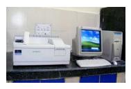
The Lambda 25 UV-visible spectrometer is provided with double beam optics, which incorporates concave holographic grating along with a proven optical design to minimize stray radiation with accurate results. The system has a noise specification of 0.0003A peak to peak, which means that 0.0003A is the lowest usable absorbance reading. The optical performance of the lambda series ensures that you will get dependable results at high and low absorbance
